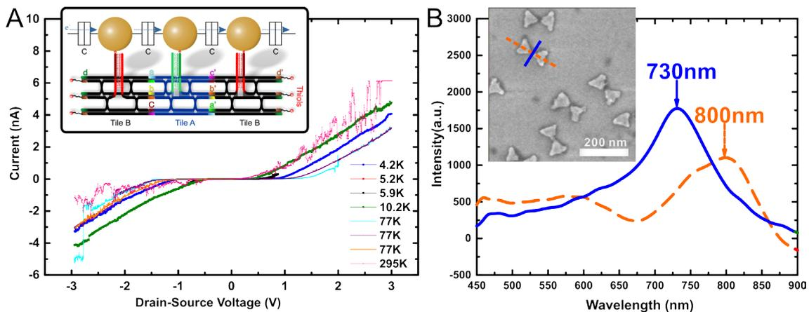
**Figure 1: (A)** IV characteristics of the pearl-like-three-AuNP-assembly (inset). The Coulomb blockade region is clearly visible from 4.2 K all the way to room temperature. **(B)** The localized surface plasmon spectra of a silver bowtie structure presented in the SEM image (inset). The blue solid and the orange dashed lines indicate the polarization angles of the excitation light as shown.
