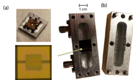
Figure 1: SiN membrane assembly, and a three-dimensional cavity
