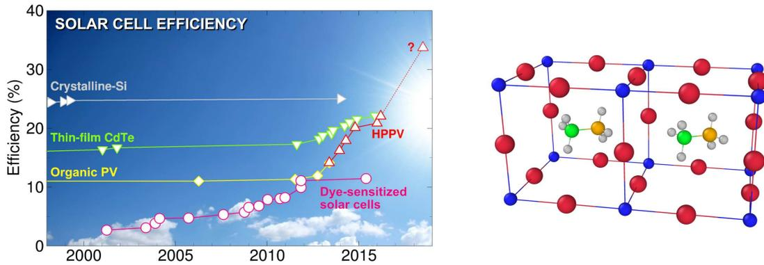
Figure 1: Left: Conversion efficiency evolution with time of different solar cell types. Right: An example of an  $\text{MA}^+$  pair configuration in neighboring  $\text{MAPbI}_3$  unit cells.
