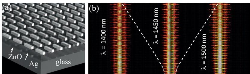
Figure 1: A metamaterial film waveguide. The geometry of the waveguide is shown in (a) and divergence-free propagation of three optical beams in the waveguide is shown in (b).
